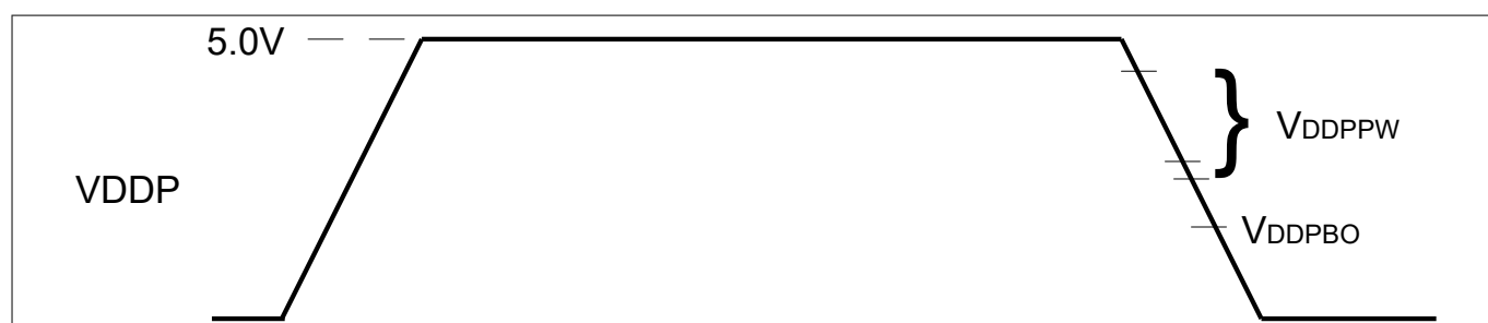
Figure 25 Supply Threshold Parameters
