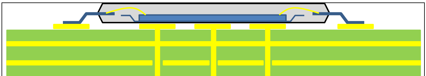
Figure 7-1: Example thermal via holes on PCB.
